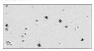
Transmission electron microscopy (TEM) image of a DeltaFil micelle suspension. Staining to increase contrast. Source: Copyright Fraunhofer IWMS, Feb. 2021, data not
