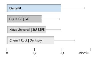
Compared to all other materials tested, DeltaFil achieves the highest fracture toughness.
